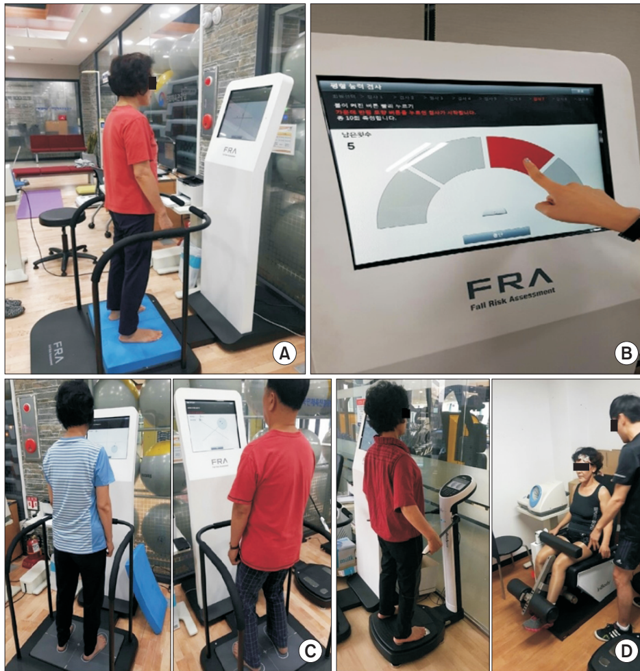
Fig. 2. Fall Risk Assessment (FRA) system and body composition analyzer. (A) A participant performing mCTSIB using the balance measuring instrument to obtain sensory score (Condition 3: on the foam surface). (B) A participant performing reaction time and latent reaction time tests by balance measuring instrument to obtain reaction score. (C) A participant performing shifting velocity test (left) and another participant performing diagonal A type target tracking test (right) using the balance measuring instrument to obtain integrated balance ability score. (D) A participant performing leg muscle mass test by body composition analyzer (left) and another participant performing leg muscle strength test by leg muscle dynamometer (right) to obtain muscular system score. mCTSIB, modified clinical test of sensory interaction in balance.
