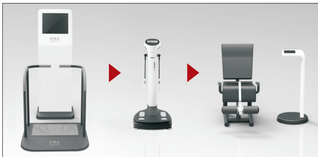
Fig. 1. Three components of Fall Risk Assessment (FRA) system: balance measuring instrument, InBody body composition analyzer, and leg muscle dynamometer.
